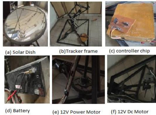
Fig. 4. Prototype Parts.
