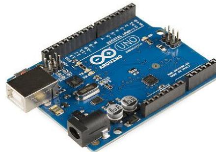
**Fig. 4.** Arduino Uno Main Controller.
